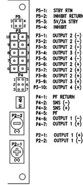
**P5:** 0.100 friction lock header mates with Molex 22-55-2041 or equivalent crimp terminal housing with Molex 71851 or equivalent crimp terminal.
